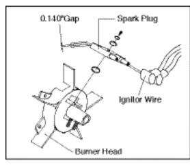
Figure 16. Removing Spark Plug
